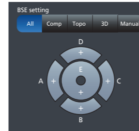
BSED graphic showing the single inner segment and four independent outer segments
