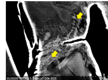
Accelerating Voltage: 15 kV, Outer segment/High angle BSE Magnification: 7,000 x, Sample: Heat resistant steel This accentuates the crystal orientation of the material
