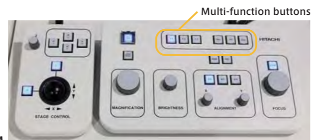
Common control panel for TEM/STEM
