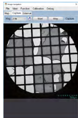
Whole view image (× 50) The desired field of view is selected from the overall image grid captured using the Whole view feature.
