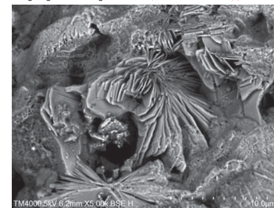
TM4000 5kV 6.2mm X5.00k BSE H Accelerating voltage: 5 kV Image signal: BSE Magnification: 5,000x Sample: Cement
